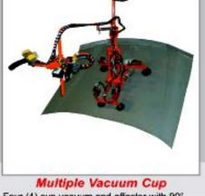
Four (4) cup vacuum end effector with 90° rotate. Transfers hood from rack to weld fixture.
